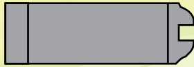
Engineered hardwood FSC Certified stave lumber core. Hardwood lumber stile and rail banding.
